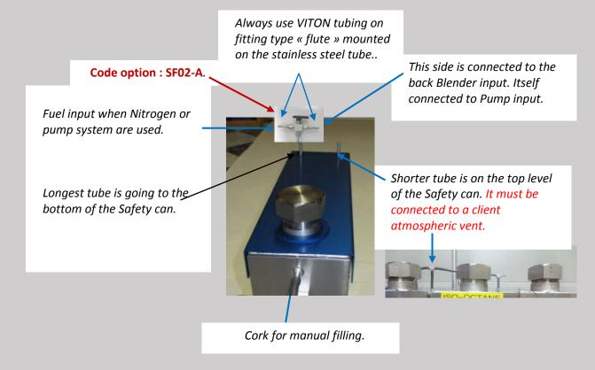
➤ Right input of the 3 ways manual valve is connected to the back blender input. This input connected to pump input. This pump will take the fuel volume required for the specific Blending.
